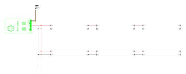
Maximum single run length 10W/M - 12M Max. Single Run Length. The Strip is 5m/reel.
