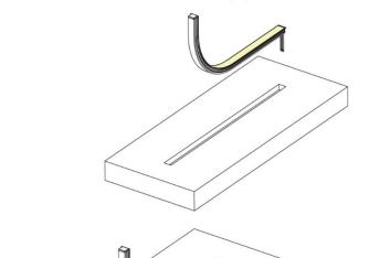
Align the light to the groove, press the glowing surface of the light, and fully embed the light into the groove
