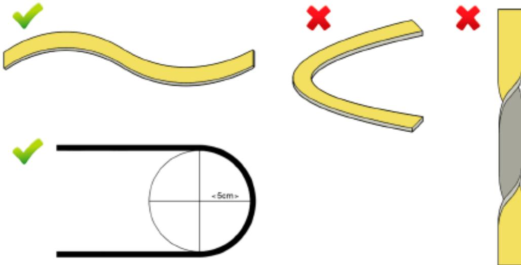
Cable and connector should never be stretched. Also, the LED strip should not be twisted. The LED strip is completely encapsulated and designed for versatile use. It can be mounted in different ways and works equally well horizontally as vertically. When mounting the LED strip, it is important that the encapsulation is kept intact.
